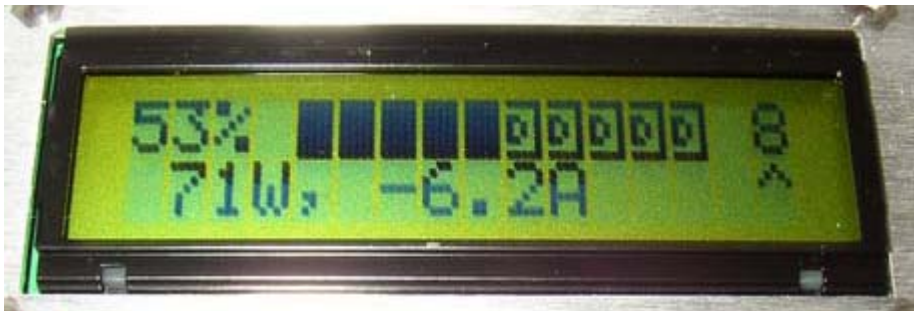
Power and Current Discharge Rate
